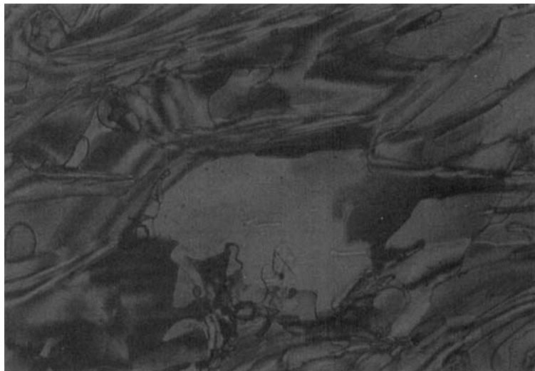
FIGURE 3 The highly ordered Smectic texture of 2a identified by optical microscope. See Color Plate. XII.
