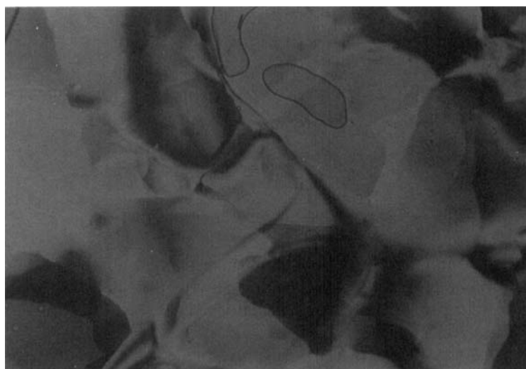
FIGURE 4 The highly ordered Smectic texture of 2c identified by optical microscope. See Color Plate. XIII.
